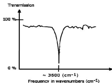
The graph above shows a spectrum in **transmission mode**. This is the **most commonly used representation** and the one found in most chemistry and spectroscopy books. Therefore we will use this representation.
